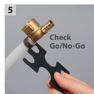
**Fitting positioning.** Insert the fitting into the pipe up to the fitting shoulder. Position the crimp ring 3-6 mm from the end of the pipe. Slightly tighten the ring with a pincers in order to avoid its displacements.
